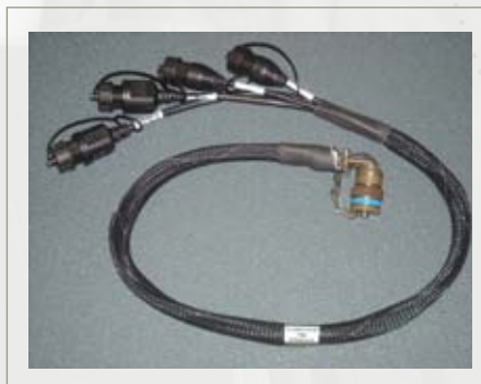
▶ Dongle cable for laptop converted to MILSPEC connectors.
