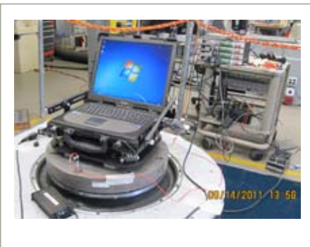
► Getac M-Series shock testing.
