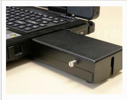
▶ Getac M-Series extended cover for special purpose PCMCIA cards.
