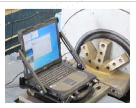
► Getac M-Series vibration testing.
