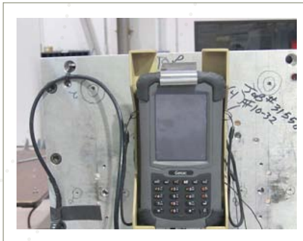
► Getac PS-Series vibration testing.
